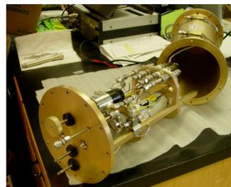
Ambient air is sampled through a standard HIMIL inlet protruding outside the aircraft boundary layer. Ambient air sample flow is controlled to 500 sccm, while the NO reagent is introduced to the reaction vessel in near-excess flow of  $\sim 4$  sccm. Gas flows as well as the reaction vessel temperature ( $35 \pm 0.1^\circ\text{C}$ ) and pressure ( $10 \pm 0.05$  torr) are all controlled at constant conditions resulting in maximum stability of the detected signal and instrument sensitivity.
