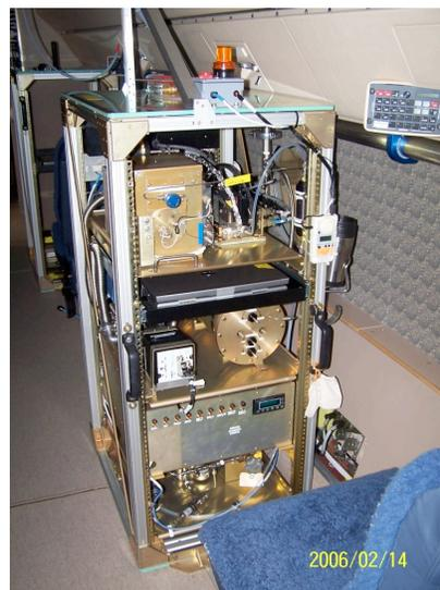
A preliminary  $\text{O}_3$  mixing ratio is transmitted to the aircraft data system, from which it is transmitted to the ground for real-time display via aeros.
