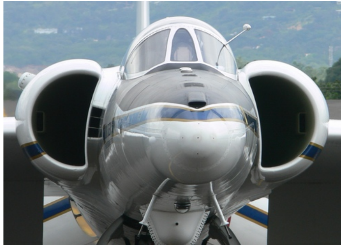
MTP located on the ER-2's right engine cheek (HDPE window just visible)
