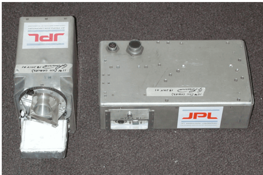
The MTP Sensor Unit (left) and Data Unit (right).
