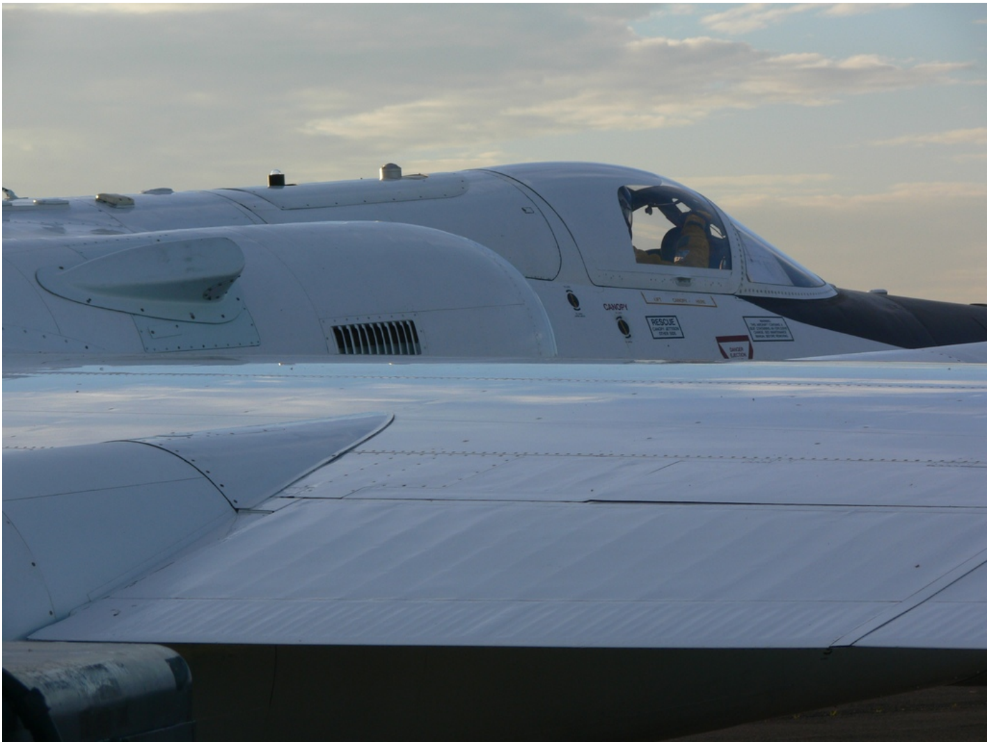
A view of the MTP fairing (left upper) on the right engine cheek of the ER-2. The Sensor Unit extends out into the fairing, and the Data Unit is mounted below it inside the engine cheek.
