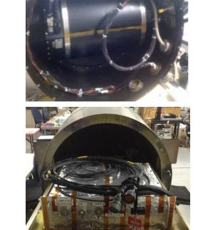
Research Scanning Polarimeter (RSP): Scanner that uses Wollaston prisms to split into polarized components. Was the airborne prototype for the Aerosol Polarimetry Sensor (APS) on the NASA Glory Mission. Principal Investigator is Brian Cairns, NASA Goddard Institute for Space Studies. See Cairns et al. 2003, Chowdhary et al, 2012 and Knobelspiesse et al., 2011.
