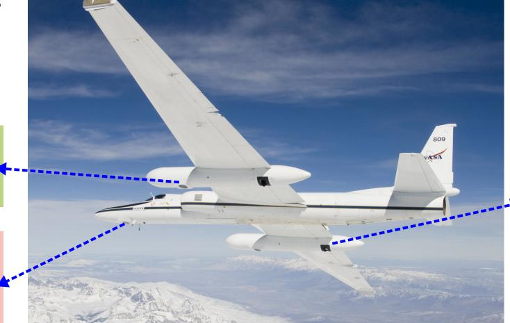
Research Scanning Polarimeter Scanner that uses Wollaston prisms to split into polarized components. Was the airborne prototype for the Aerosol Polarimetry Sensor (APS) on the NASA Glory Mission. Principal Investigator is Brian Cairns, NASA Goddard Institute for Space Studies. See Cairns et al., 2003, Chowdhary et al, 2012 and Knobelspiesse et al., 2011.
