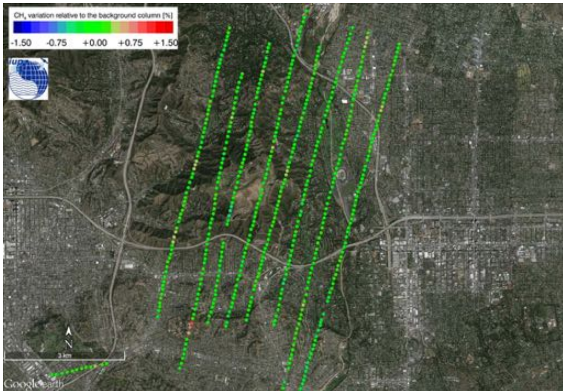
Figure 89: Normalized column averaged dry air mole fraction of CH_4 of the MAMAP remote sensing sounding of the Scholl Canyon Landfill on 2014-08-27.
