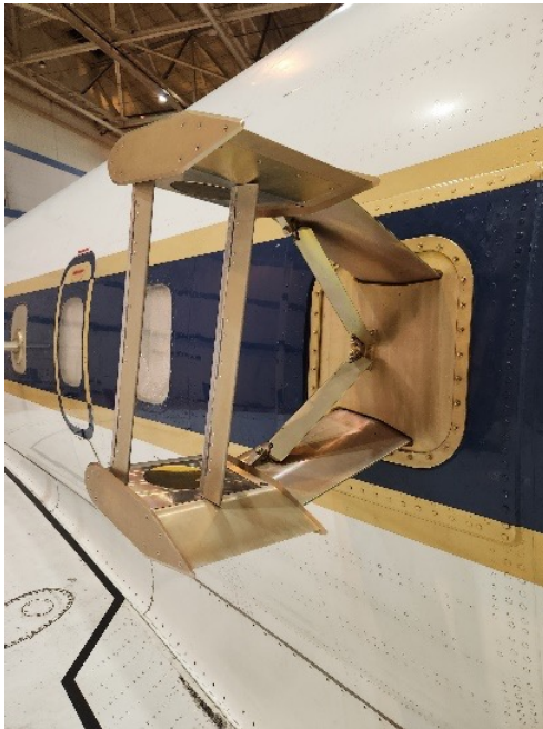
Figure 45. The OPALS instrument, as seen from the exterior of the DC-8, showing the metering rods and spherical mirrors. Photo credit: Adam Webster
