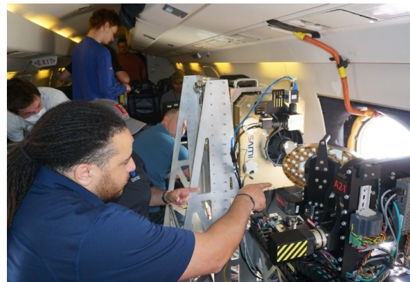
Figure 58. HORIS team members Carey Scott (NASA) and Tait Pottebaum (OKSI) discussing installation of SAMI on NASA 522. Photo credit: Mary Emmerson
