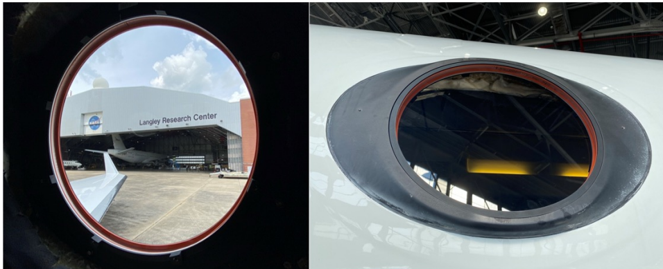
Figure 59. Inside (a) and outside (b) views of fused silica optical windows. Photo credit: Arianna Haven
