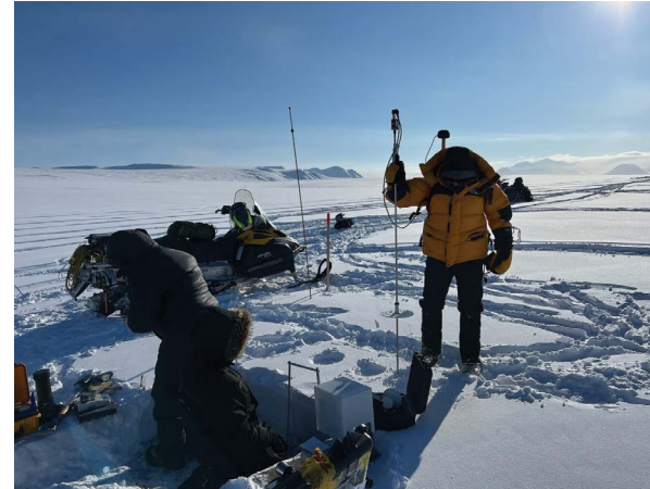
Measuring snow profile information and depth at the SnowEx Upper Kuparuk-Toolik tundra site. Photo: S. Stuefer
