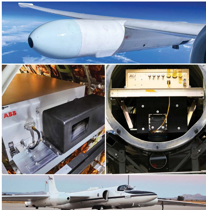
Top: Photo from cockpit of starboard wing pod during flight. Middle: SHOW (L) and ALI (R) integrated in the wing pod before flight. Bottom: NASA ER-2 aircraft during the HAWC campaign. Photo: P. Loewen
