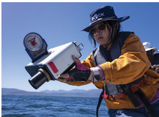
BioSCape PI Jinghui Wu (Columbia U.) taking radiometric measurements of coastal ocean waters in South Africa. Photo: O.Whitehead
