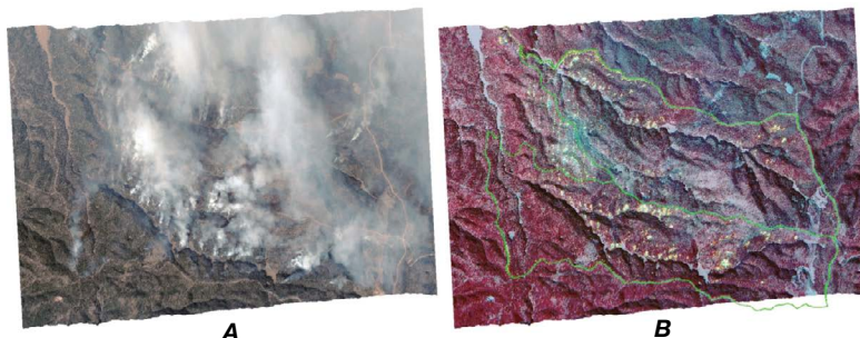
Side-by-side views of the same burn site in the Kaibab Plateau, AZ, taken October 20-21, 2023. These images demonstrate the multifaceted capabilities of the MASTER instrument. The natural color composite (A) shows the burn area as it would appear to the human eye, replete with smoke during the day, and the glow of the active fire at night (C). The false-color image (B) is a thermal and short-wave infrared rendition, penetrating the smoke and portraying the active fire lines.
