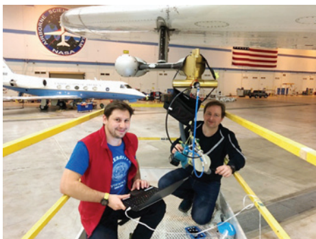
University of Vienna CAPS instrument on DC-8 wingtip being checked out by (L-R) Max Dollner and Nickolaus Foelker during ATom-4 integration.
