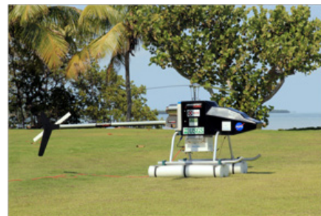
Vision II UAS carrying NovaSol hyperspectral imager
