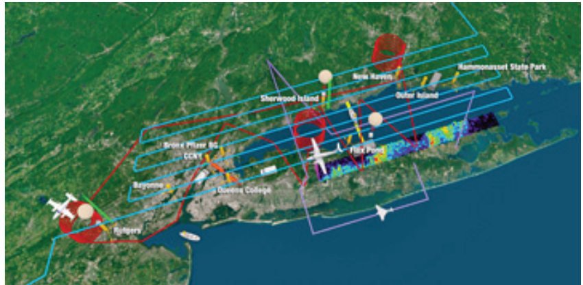
Flight tracks of various aircraft during LISTOS. Blue tracks are a depiction of those flown by the B-200. Red spirals were flown by a UMD Cessna. Green beams are ground-based ozone lidars, orange tripods are Pandora remote sensing stations, and white balloons indicate the ozone sonde locations.
