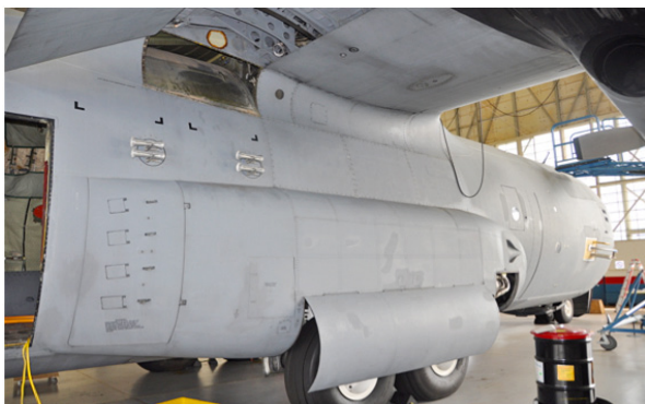
C-130 fitted with probes in the forward window for the NAAMES mission.
