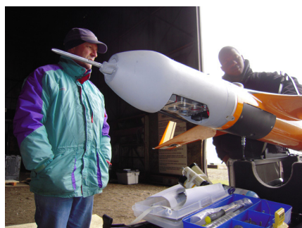
A UAF ScanEagle with the CU air-deployed microbuoy system installed.
