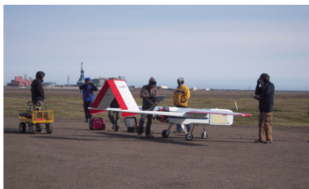
The NASA SIERRA undergoing ground checks. One of the three available payload "nose bays" is installed.
