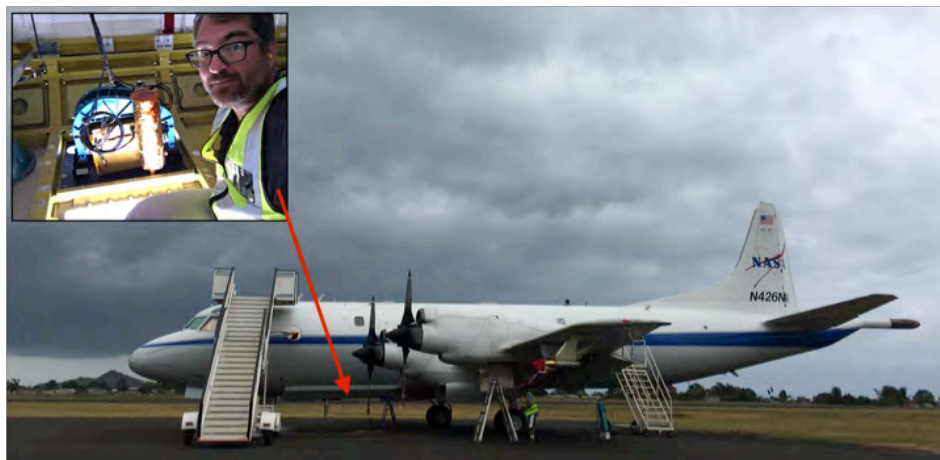
FIGURE 35 The NASA P-3 aircraft on the ground in São Tomé. The Research Scanning Polarimeter (RSP) is located in the "bomb bay," in the fuselage just forward of the engines.
