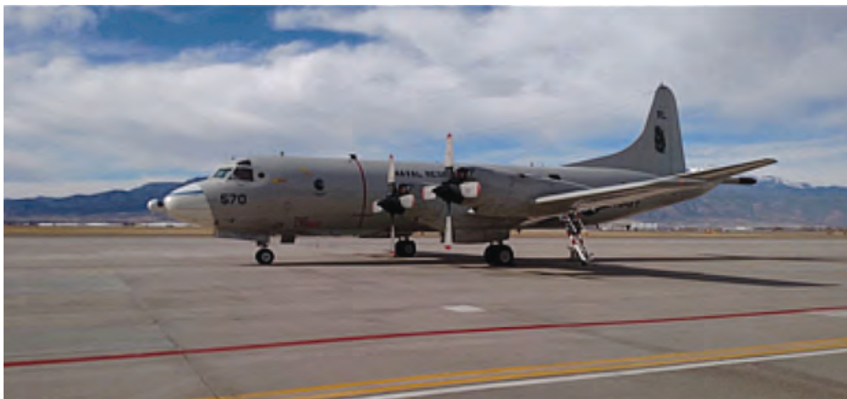
FIGURE 24 NRL P-3 (VXS-1 squadron, Pax River) deployed at Peterson AFB for SnowEx. Visible are NASA P-3's nose housing CAR and the tail & nadir housings for the SnowSAR.
