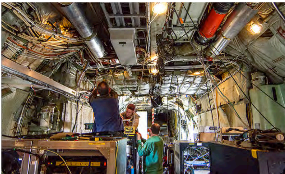
FIGURE 39 Inside the C-130 cargo area during NAAMES. Wires, conduits and specialized hardware take up nearly every inch of the cabin area.
