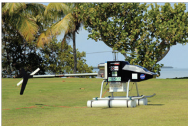
Figure 26. Vision II UAS carrying NovaSci hyperspectral imager.
