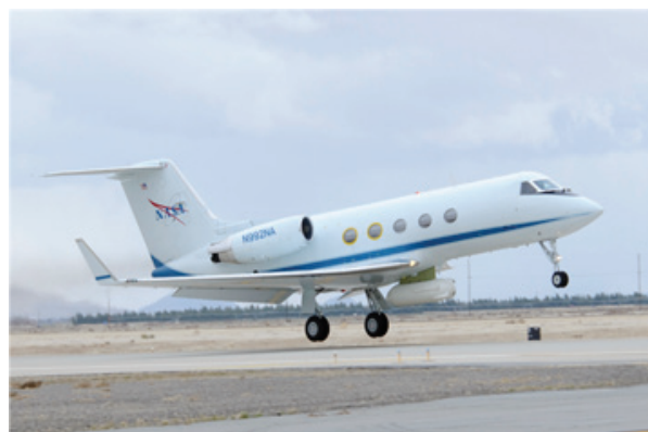
Figure 36. JSC G-III carrying AirMOSS in SAR pod.
