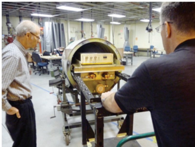
Figure 23. During a test phase for the PODEX experiment, engineers and the crew at Dryden Aircraft Operations Facility loaded the Research Scanning Polarimeter into the “superpod,” for placement under the wing of the ER-2.
