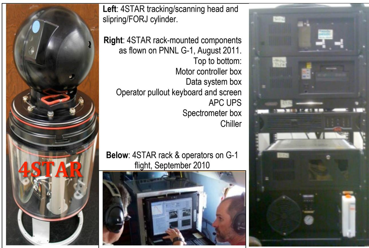
4STAR has made several test flights on the PNNL G1, and its full capabilities are still being developed. When it achieves those full capabilities, we expect that, in addition to AATS-like direct-beam measurements of aerosol optical depth (AOD) and water vapor,
