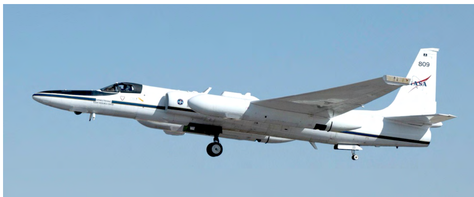
Figure 24. NASA's ER-2 high-altitude aircraft carrying the AirMSPI-2 science instrument payload in the nose cone during MAIA science and launch preparation flights in April 2025. Credit: Carla Thomas/ NASA AFRC.
