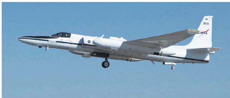
Figure 56. NASA's ER-2 high-altitude aircraft carrying the AirMSPI-2 science instrument payload in the nose cone during MAIA science and launch preparation flights in April 2025. Credit: Carla Thomas/NASA AFRC
