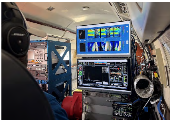
Figure 44. NASA High Altitude Lidar Observatory (HALO) Principal Investigator, Amin Nehrir, looks on as the backscatter signal spike from the contrail becomes visible on the lower monitor. Credit: NASA
