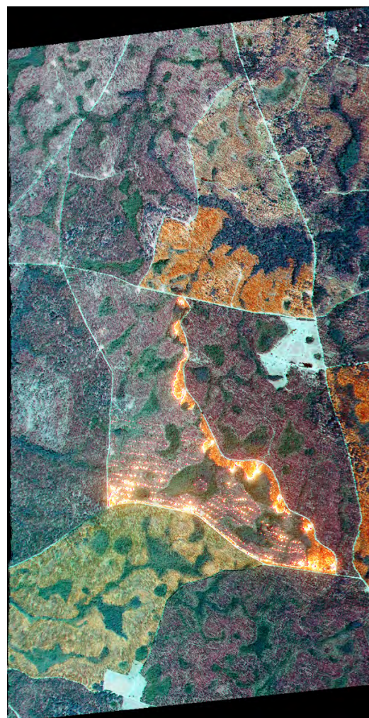
Figure 17. Fire progression and ignition pattern captured by the MASTER sensor during a prescribed burn at Fort Stewart-Hunter Army Airfield on April 16, 2025. The image is a geocorrected false color composite showing the active fire as bright yellow and burning or recently burned areas as red and orange. Credit: ARC ASF MASTER Team/NASA
