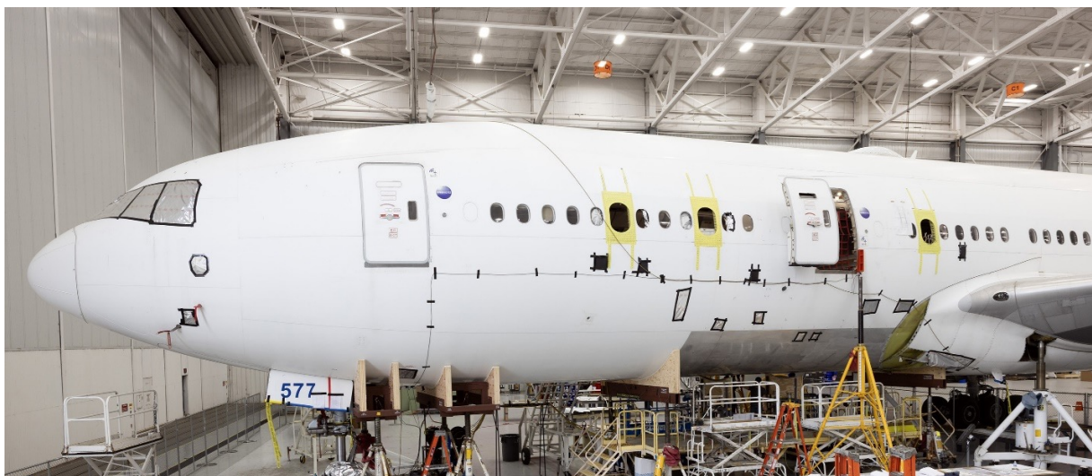
Figure 68. B777 showcasing work in progress on window modification. Credit: L3 Harris
