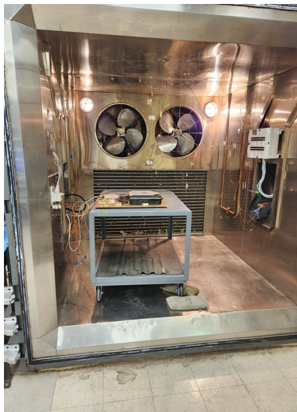
Figure 77. Soxnav flight hardware inside one of AFRC's environmental test chambers. This chamber exposed the flight hardware to extremes of heat, cold, and altitude. Credit: John Sonntag
