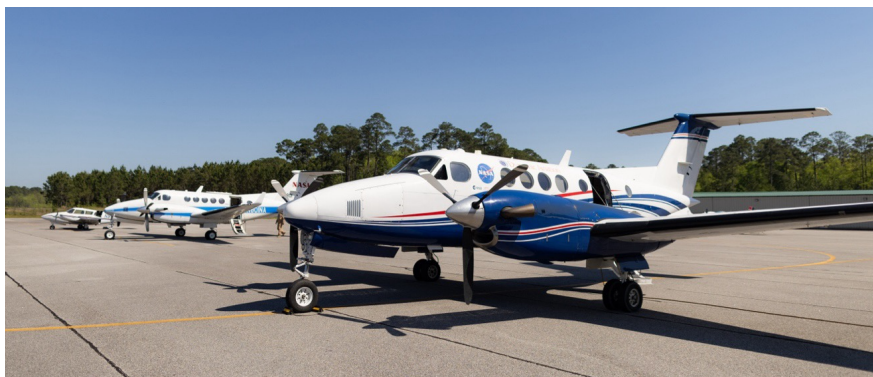
Figure 19. Three crewed aircraft outfitted with five total instruments sit on the tarmac at Fort Stewart Hunter Army Airfield. From front to back: a Dynamic Aviation B-200 carrying AVIRIS-3, NASA B-200 carrying the FireTIRS and MASTER sensors, and Trident Sensing's Piper Twin Comanche carrying the TACFI-RS sensor. Credit: Milan Loiacono/NASA
