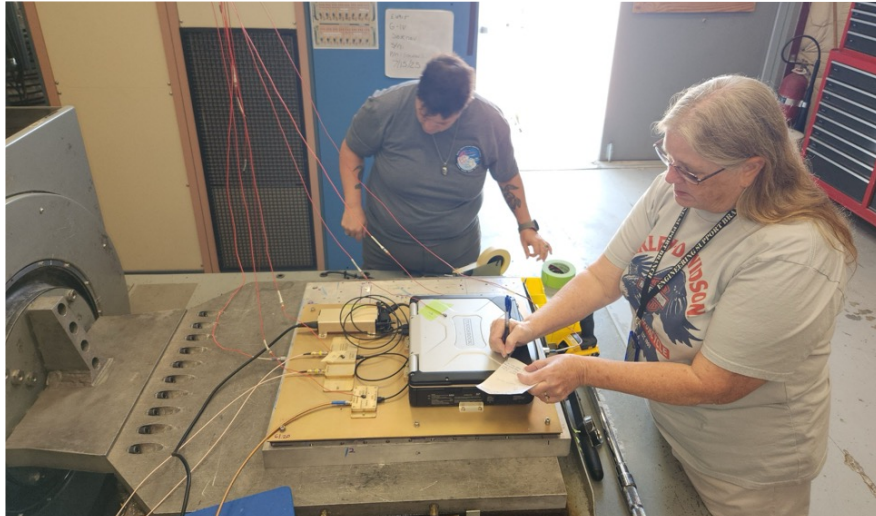
Figure 75. AFRC's Cryss Puntenev (left) and Karen Estes (right) preparing one of the Soxnav flight hardware assemblies for vibration testing. Red cables are accelerometer leads, which enable the response of the hardware to be monitored at many discrete points. Credit: John Sonntag
