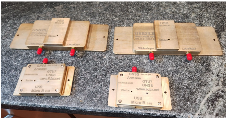
Figure 76. Production Soxnav radio-frequency electronics modules (top) and GNSS modules (bottom). Credit: John Sonntag
