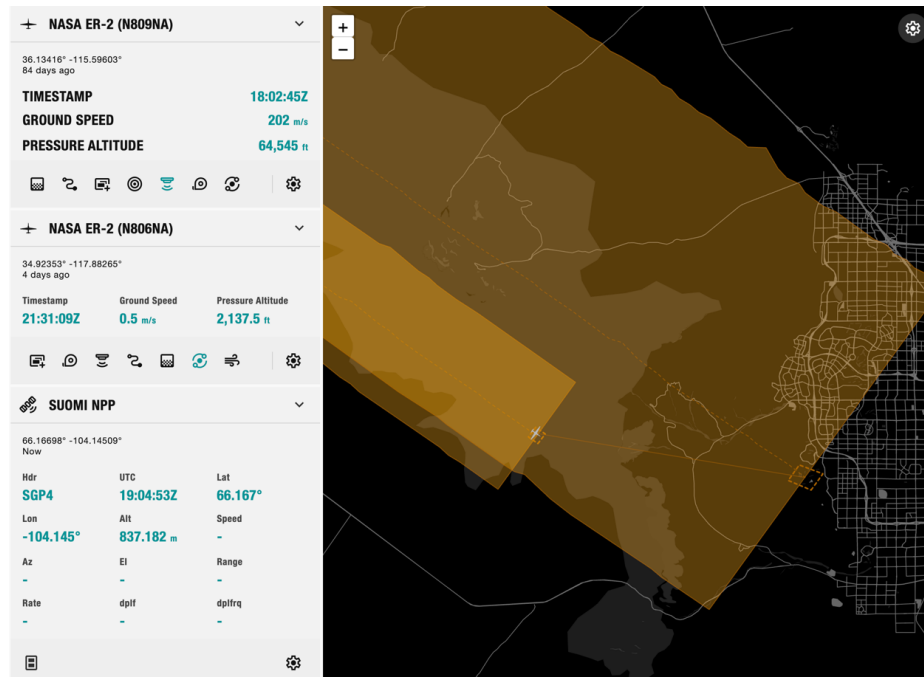
Figure 80. New advanced dynamic swath overlay depicting a nadir and off-nadir sensor configuration. Credit: Aaron Duley/NASA ARC
