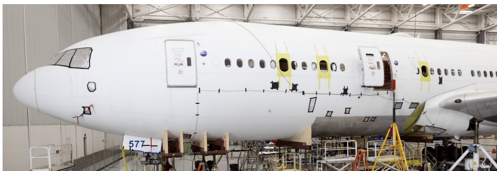
Figure 55. B777 showcasing work in progress on window modification. Credit: L3 Harris
