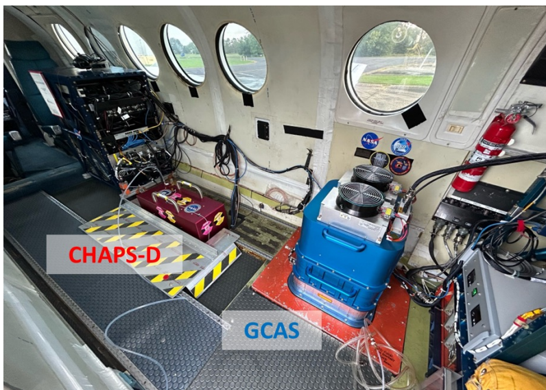
Figure 29. CHAPS-D and GCAS (GSFC) integrated on B-200. Credit: William Swartz/JHU/APL
