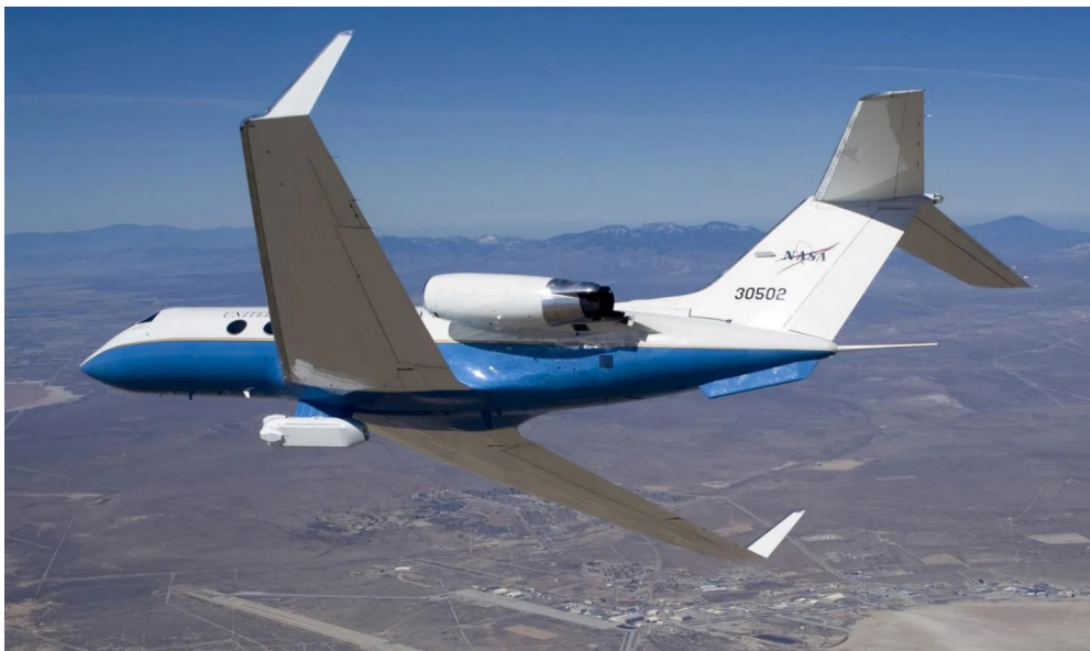
Figure 59. The Uninhabited Aerial Vehicle Synthetic Aperture Radar (UAVSAR) underbelly pod is in clear view as NASA's Gulfstream III research aircraft banks away over Edwards Air Force Base, California.
