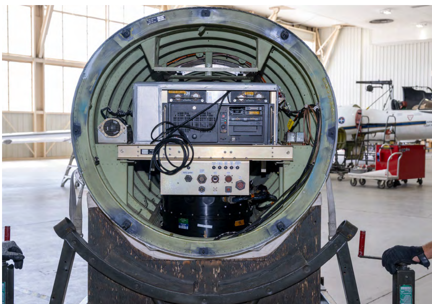
Figure 23. AirMSPI-2 installed in the nose cone of NASA's ER-2 high-altitude aircraft at Armstrong Flight Research Center. April 2025 marked its first successful science deployment, collecting multi-spectral data critical for aerosol and surface studies. Credit: Genaro Vavuris/ NASA AFRC.
