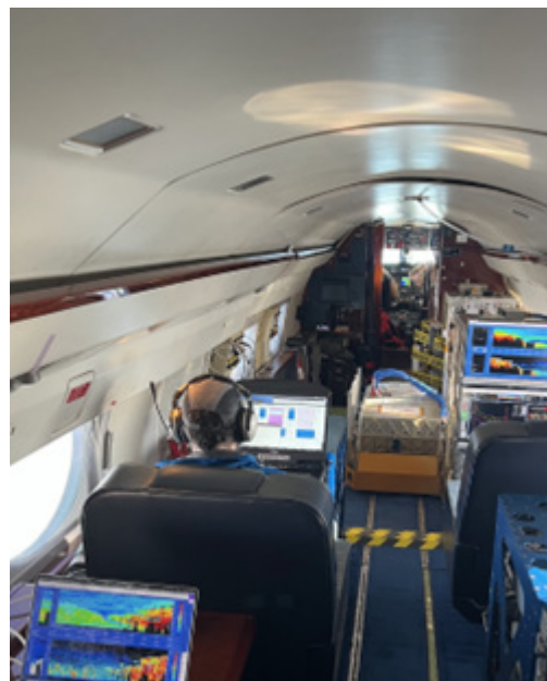
Figure 8: The NURTURE payload inside the NASA G-III on Research Flight 03. The HALO lidar and CloudCube radar can be seen in the background with their respective instrument operator racks. In-situ trace gas and Mission Science stations are in the foreground. Credit: Amin Nehrir / NASA LaRC
