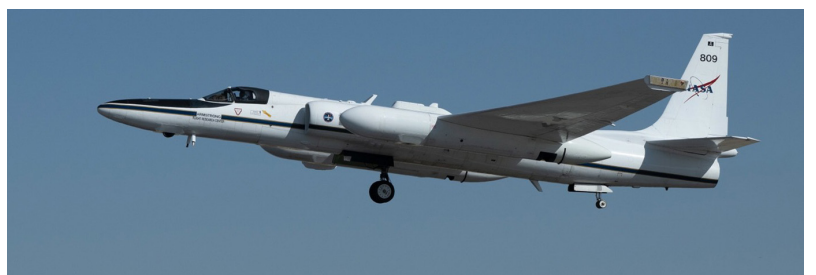
Figure 6: NASA's ER-2 aircraft carrying the AirMSPI-2 science instrument payload in the nose cone during MAIA science and launch preparation flights. Credit: Carla Thomas / NASA AFRC.
