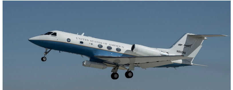
Figure 14. NASA's C-20A takes off from NASA's Armstrong Flight Research Center in Edwards, California, on April 29. The aircraft carries the Uninhabited Aerial Vehicle Synthetic Aperture Radar (UAVSAR), used to study the San Andreas Fault in Central California and support validation of a hazard-monitoring satellite's radar. The flight series will also help scientists refine earthquake models. Credit: Jim Ross / NASA
