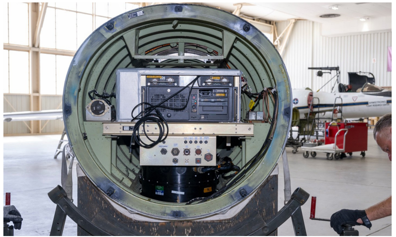
Figure 5: AirMSPI-2 installed in the nose cone of NASA's ER-2 high-altitude aircraft at Armstrong Flight Research Center. April 2025 marked its first successful science deployment, collecting multi-spectral data critical for aerosol and surface studies. Credit: Genaro Vavuris / NASA AFRC.
