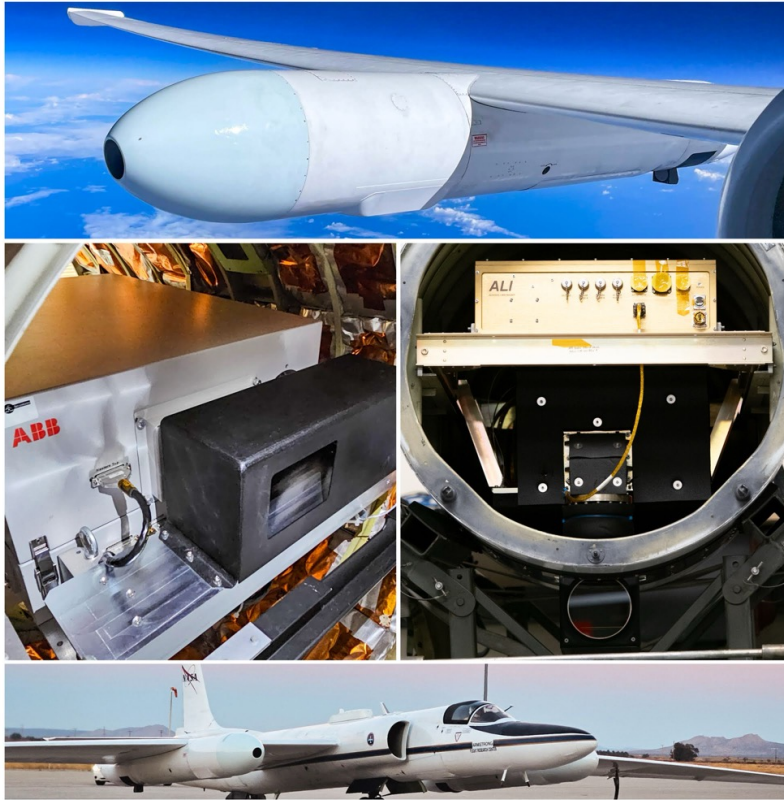
Figure 62. Top: Photo from cockpit of starboard wing pod during flight. Middle: SHOW (L) and ALI (R) integrated in the wing pod before flight. Bottom: NASA ER-2 aircraft during the HAWC campaign. Credit: P. Loewen
