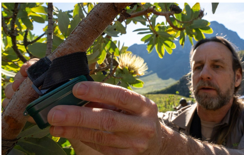
Figure 12. BioScape Science Team member Andrew Turner (CapeNature) deploying an Audiomoth acoustic logger in South Africa. Credit: Jeremy Shelton
