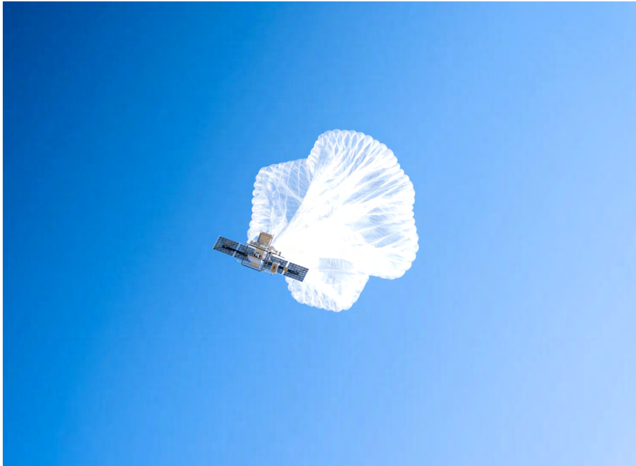
Figure 63. The Aerostar stratospheric station-seeking balloon is released, carrying the USFS/NASA communications and imaging payload. The balloon appears deflated because it will expand as it rises to higher altitudes where pressures are lower. Credit: Austin Buttlar/ Colorado Division of Fire Prevention and Control Center of Excellence for Advanced Technology Aerial Firefighting
