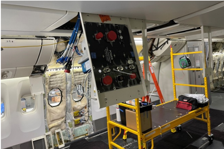
Figure 101. B777 cabin experimenter station interface panel. Credit: NASA
