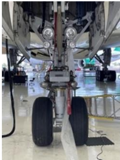
New landing gear installed on the NASA B777 at Citadel Completions in Lake Charles, LA. Credit: Derek Rutovic / NASA
